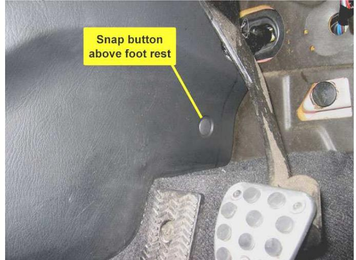
**Photo 5 – Remove snap that gets stuck in foot well wall**
